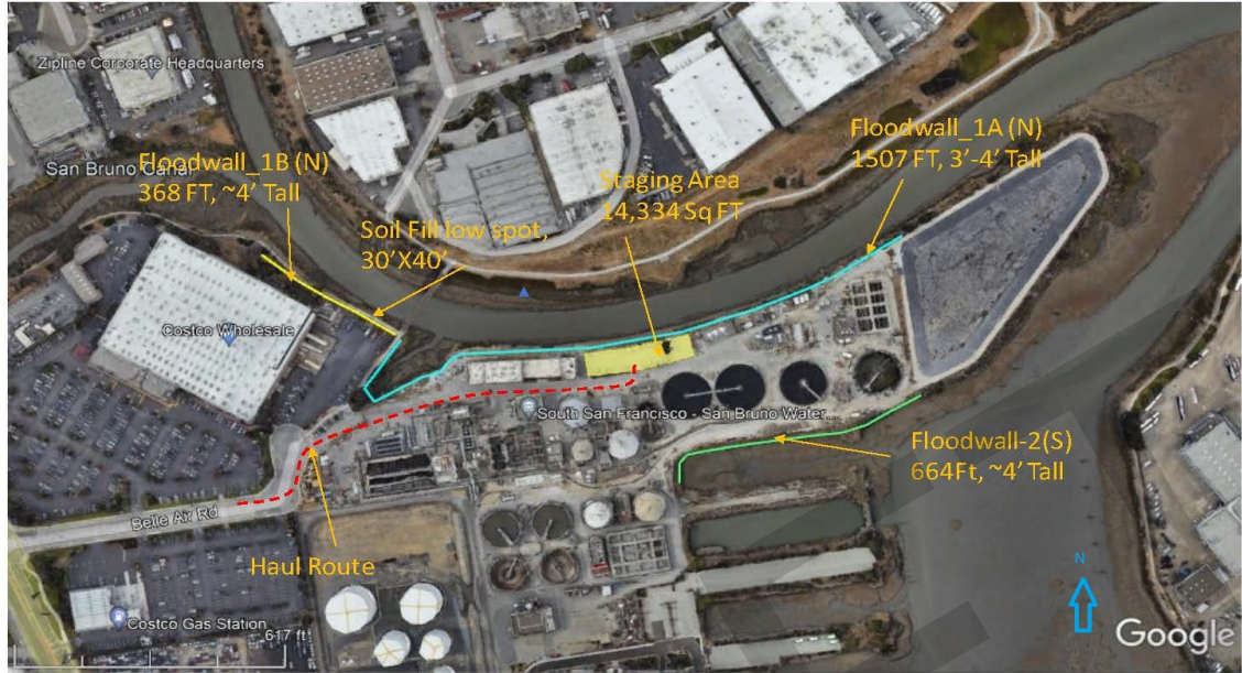
LOWER COLMA CREEK TSP - FLOODWALLS 1A, 1B (N) & 2(S)
